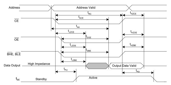
Figure 7. SRAM Read Cycle #2:  $\overline{\text{CE}}$  and  $\overline{\text{OE}}$  Controlled [3, 15, 19]
